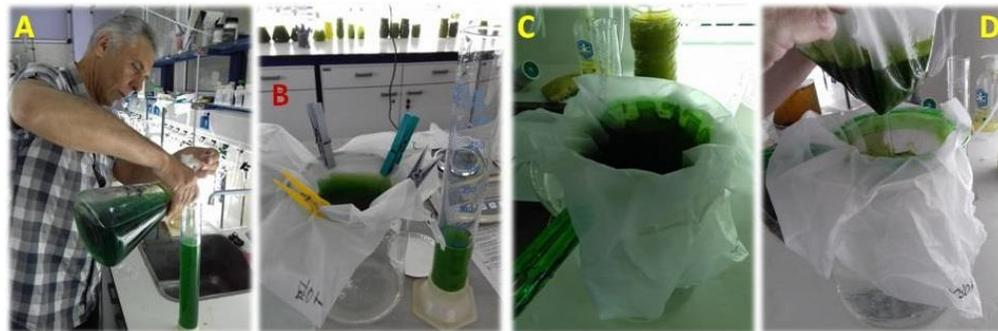
Figure 35. Process of concentrating the *Phormidium* culture (A) by pouring it into a 100  $\mu\text{m}$  planktonic mesh net (B) and draining the culture (C) so that only a dense mass of *Phormidium* filaments remains in the net (D).
